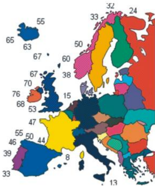
Figure 3.19: Wave power (in kW/m of wave crest length) in European waters (from CRES 2002).
